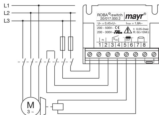
DC-side switching means **short brake engagement times (e.g. for EMERGENCY STOP operation)**; but louder switching noises will occur.
