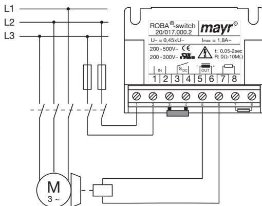
AC-side switching means **low-noise switching**; however, the brake engagement time is longer (approx. 6 – 10 times longer than with DC-side switching), use for non-critical braking times.
