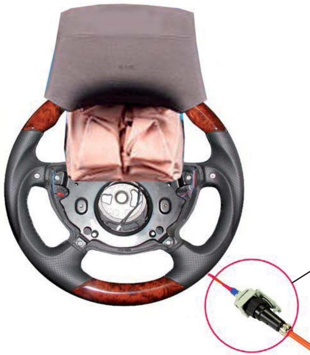
Fig. 1: Measuring forces involved in inserting and withdrawing airbag connectors with a male test connector, which transmits the forces directly to the sensor Type 9203.
