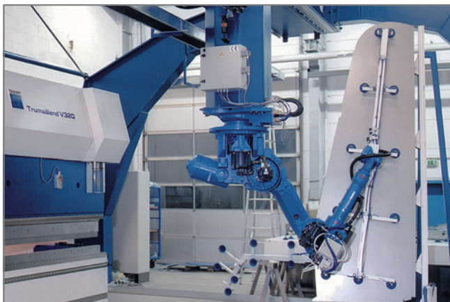
Flat suction pads SAF being used for handling sheet metal parts
