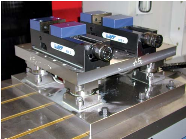
Fig. 1: Measuring platform for acquiring cutting forces, built with 3-component quartz force links
