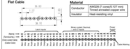
Note 1: Specify a cable length code (0.5: 500 mm, 1: 1000 mm, 2: 2000 mm, 3: 3000 mm, 4: 4000 mm, 5: 5000 mm) in place of  $\Box$  in the Part No. Note 2: As a strain relief is supplied with the connector on the display unit, the actual cable length reduces by 10 mm from the normal length.
