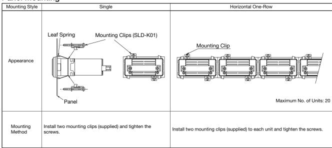
Note: Mounting Clips require only light tightening (0.34±0.04 N • m).
