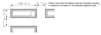
Note: Two Mounting Clips (SLD-K01) are supplied with each display unit. (Tightening torque: 0.35 N·m) Two Leaf Springs for vertical mounting are also supplied.
